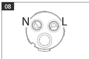
Connect the cables correctly to the core.
