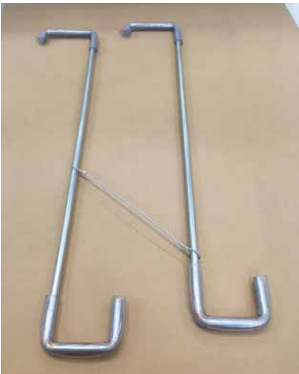
19 - Supplied manual radiator lifting tool
