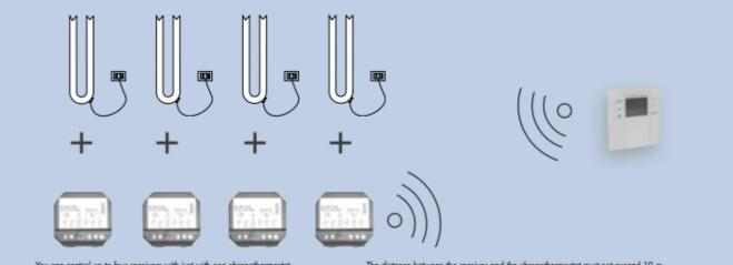
You can control up to four receivers with just with one chronothermostat.
