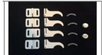
**Step 1:** You will see a small indentation on the underside of one of the collectors and this indicates where the diverter is situated. When fitting the radiator the indentation must be placed at the bottom to ensure that the water will flow correctly.
